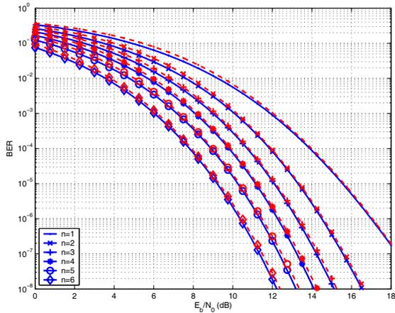
Fig. 2. Performance of the  $n$ -th best user among  $N = 6$  users under lognormal scintillation. Solid and dashed lines correspond to the exact and approximate BER's, respectively.
