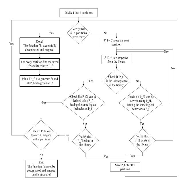
Figure 13: Improved decomposition of 5-and-less-input functions
