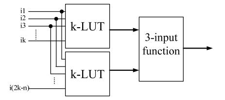
Figure 22: Configuration with k-input LUTs and n shared inputs
