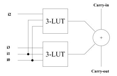
Figure 9: Logic cell in a 3-3-2 structure
