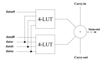
Figure 3: Logic cell in a 4-4-3 structure
