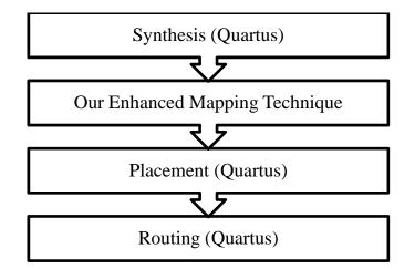
Figure 14: Modified flow of compilation phases
