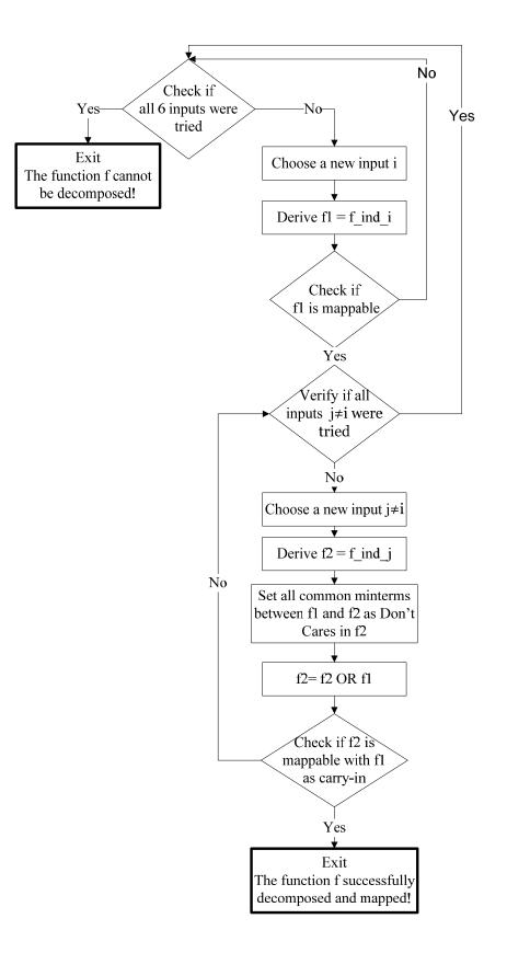
Figure 11: 6-input function decomposition and mapping process
