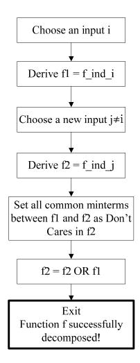
Figure 10: 6-input function decomposition process
