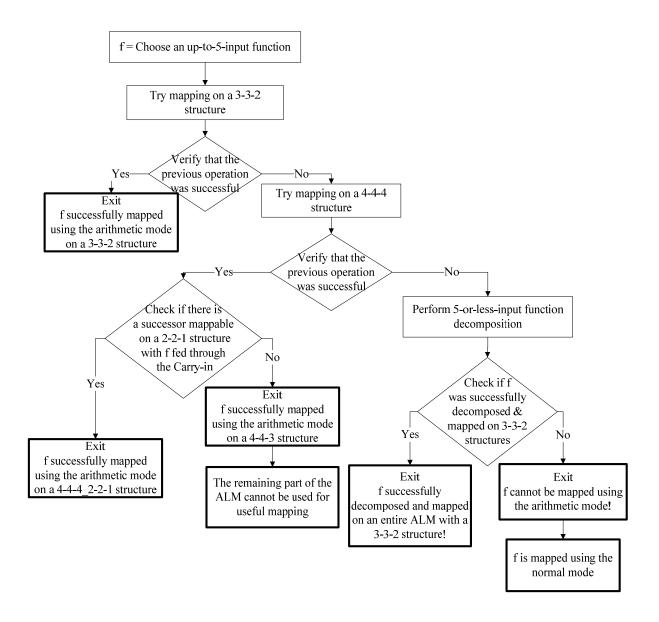
Figure 18: 5-or-less-input functions mapping process
