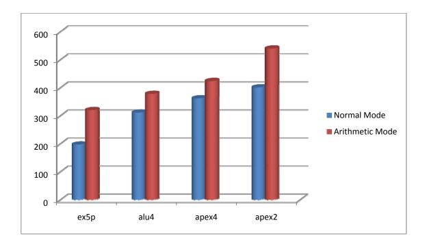
Figure 27: Representation of the overhead in used ALMs for EMTII
