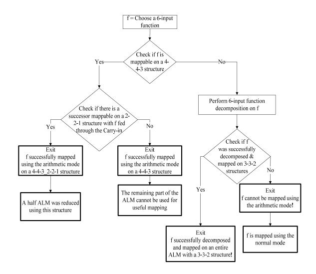
Figure 17: 6-input functions mapping process
