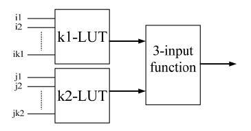
Figure 21: Configuration with variable-input LUTs (k1, k2)
