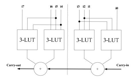
Figure 8: Carry propagation in arithmetic mode
