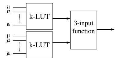
Figure 20: Configuration with k-input LUTs
