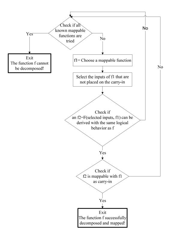
Figure 12: 5-and-less-input functions decomposition and mapping process
