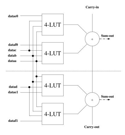
Figure 1: Adaptive Logic Module (ALM) in Arithmetic mode
