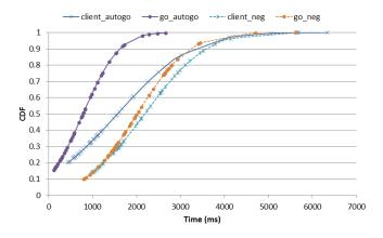
Fig. 5. Two devices P2P group formation time comparison
