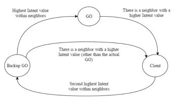
Fig. 2. Device state machine
