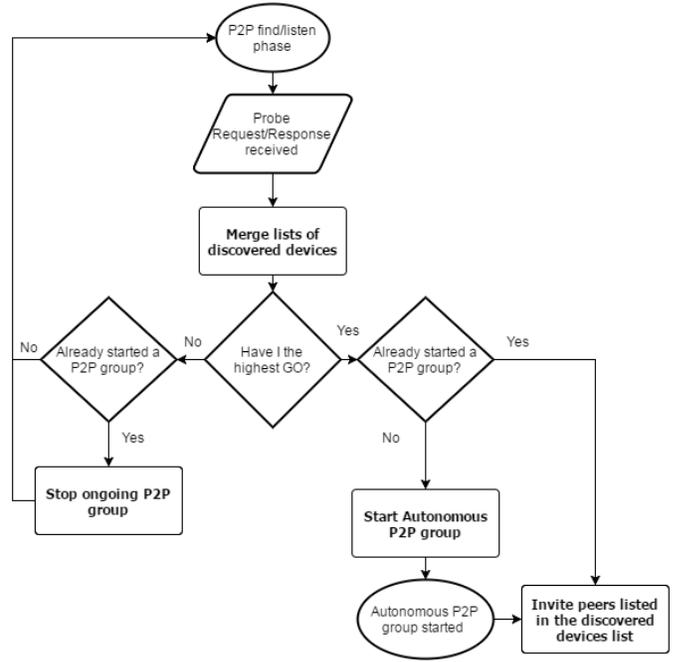
Fig. 1. Devices state diagram with the proposed P2P group formation method
