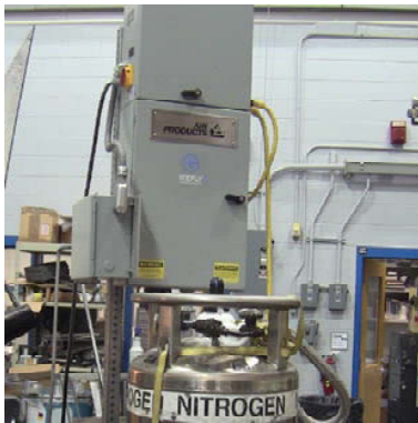
Fig. 2. Liquid Nitrogen cryogenic cooling setup with the storage tank can be seen at the bottom of picture
