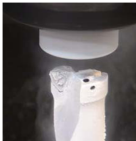
Figure 3. Photograph showing the cryogenically cooled indexable drill engaged with Mg work.
