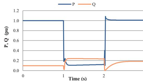
Fig. 3. The P, Q response of the inverter based DG model to a short circuit
