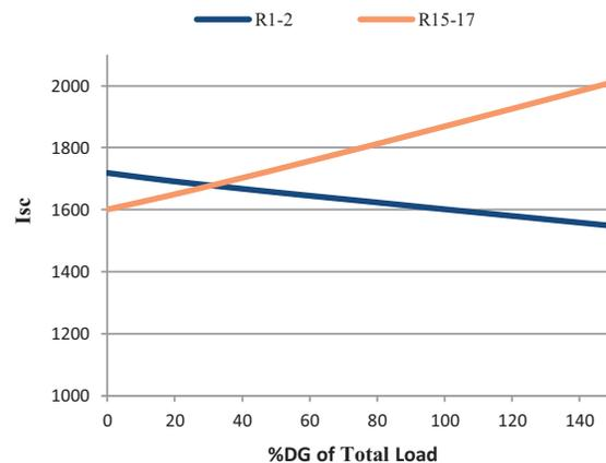
Fig. 6. Effect of Inverter Based DG on Relay Coordination
