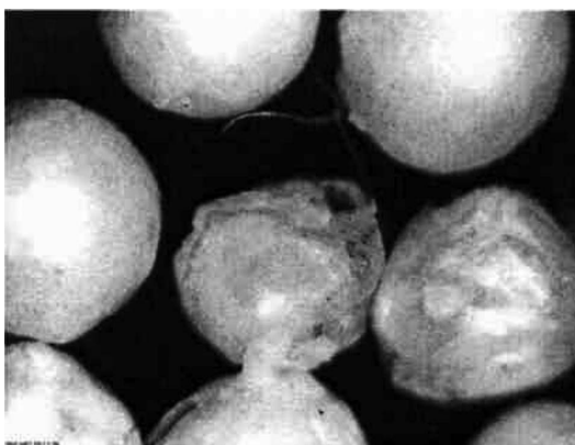
Figure 8. Electron micrograph of microspheres after dissolution at 37°C, pH 8.6, 8 mL/min flow rate.
