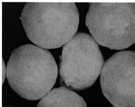
Figure 11. Electron micrograph of microspheres after dissolution at 37°C, pH 7.6, 8 mL/min flow rate and containing 0.1% sodium lauryl sulfate.
