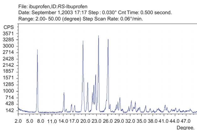
**Figure 2.** X-ray powder diffraction of pure ibuprofen.
