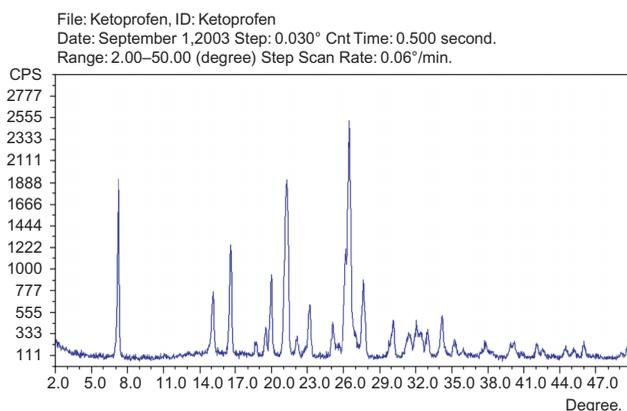
**Figure 3.** X-ray powder diffraction of pure ketoprofen.
