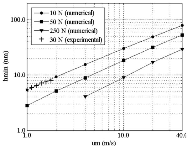
Fig.1 Orders of magnitude for minimum film thickness in lubricated contacts in nowadays industrial applications. From experimental and Finite Element approach in [1]
