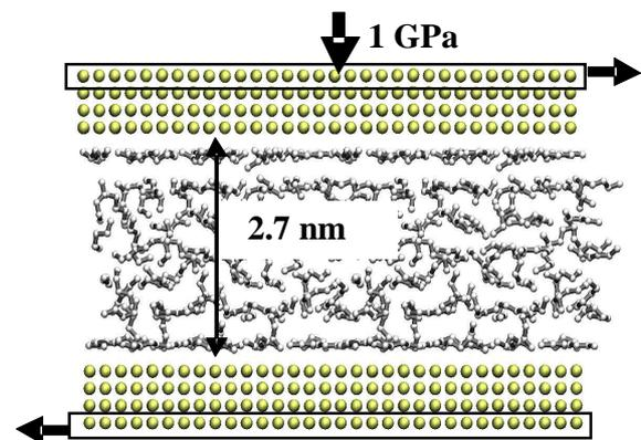
Fig.2 Snapshot of a 3D Molecular Dynamics simulation of an infinitely long lubricated contact (periodic boundary conditions). Surfaces: gold, lubricant: pentane.
