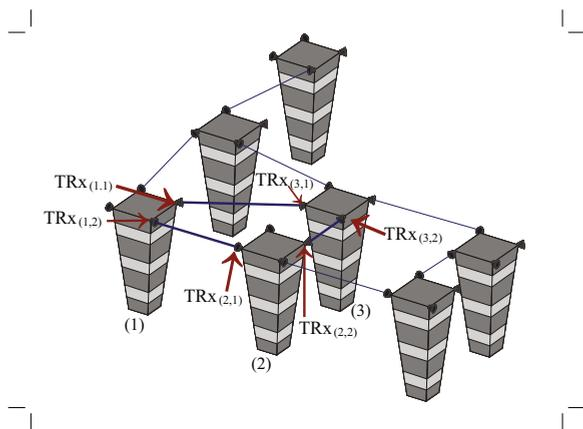
**Fig. 1.** An example of a mesh FSO network. Cooperation is proposed among the transceivers on buildings (1), (2) and (3) where the transceivers on building 2 can help in transmitting an information message from (1) to (3). Note how, given the non-broadcast nature of FSO transmissions, one couple of FSO transceiver units is dedicated for each link.
