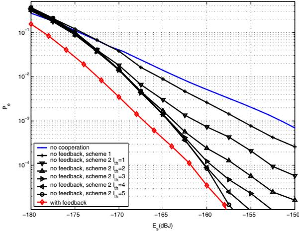
**Fig. 5.** Performance of 4-PPM in the presence of background radiation with  $P_b T_s / Q = -185$  dBJ and  $\beta_1 = \beta_2 = 4$ . Scheme 2 is applied with no energy reuse
