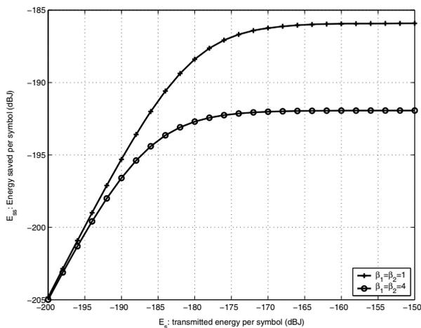
**Fig. 4.** Energy saved when scheme 2 is applied (with no energy reuse) in the absence of background radiation
