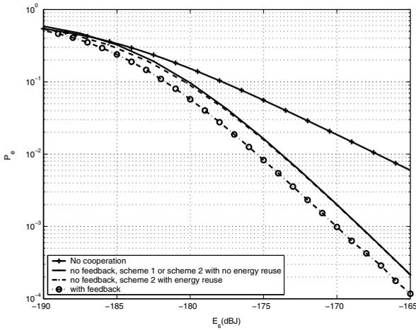
**Fig. 3.** Performance of 4-PPM in the absence of background radiation. In this figure, we fix:  $\beta_1 = \beta_2 = 4$ .
