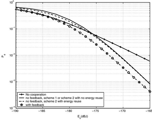
**Fig. 2.** Performance of 4-PPM in the absence of background radiation. In this figure, we fix:  $\beta_1 = \beta_2 = 1$ .
