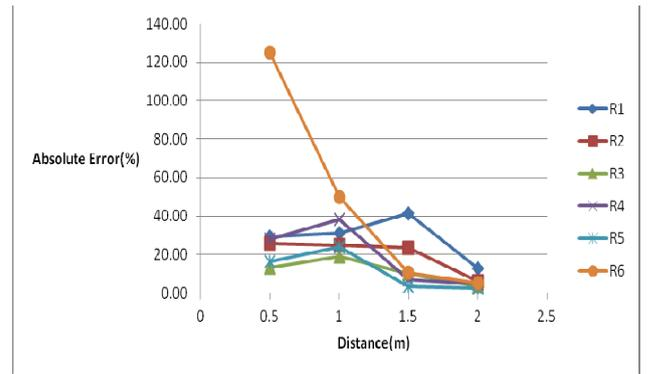
**Figure 8: Variation of Absolute Error as a function of distance at 50 km/hr (Method 2)**
