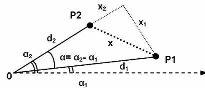
**Figure 1: Speed Calculation Algorithm [4]** the speed of the vehicle can be determined using the following equations:
