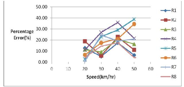
**Figure 10: Variation of Absolute Error as a function of speed**
