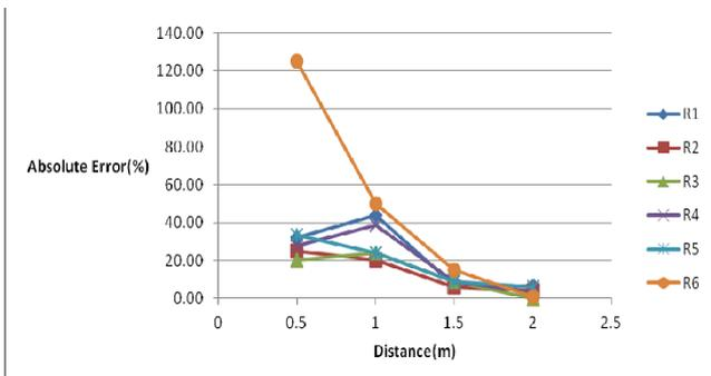
**Figure 7: Variation of Absolute Error as a function of distance at 50 km/hr (Method 1)**
