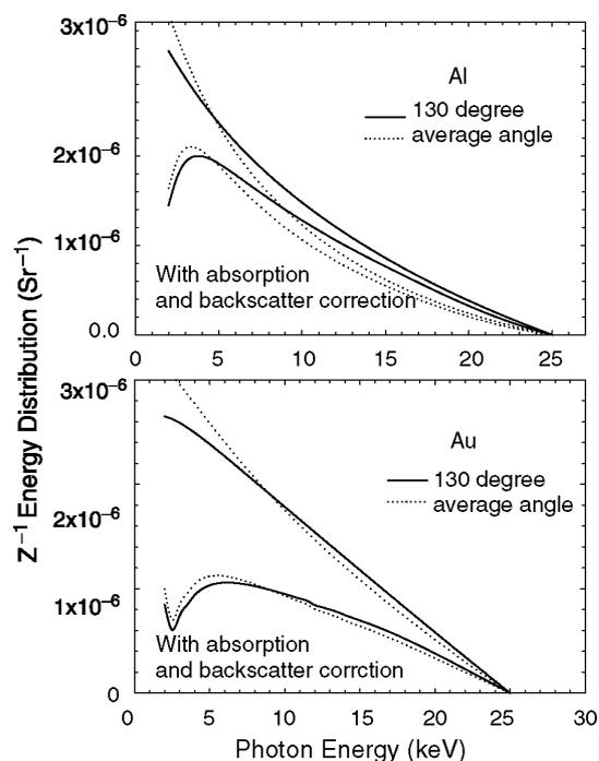
**Figure 3.** X-ray energy distribution from Eqn (4) for 130° emission angle (solid line) and for average emission angle (dotted line) for Au and Al at 25 keV. In each plot the upper curves are the energy distribution computed using the KQP thin-target cross-sections<sup>5</sup> without correction for electron backscattering and self-absorption. The lower curves include corrections for self-absorption and backscattering.
