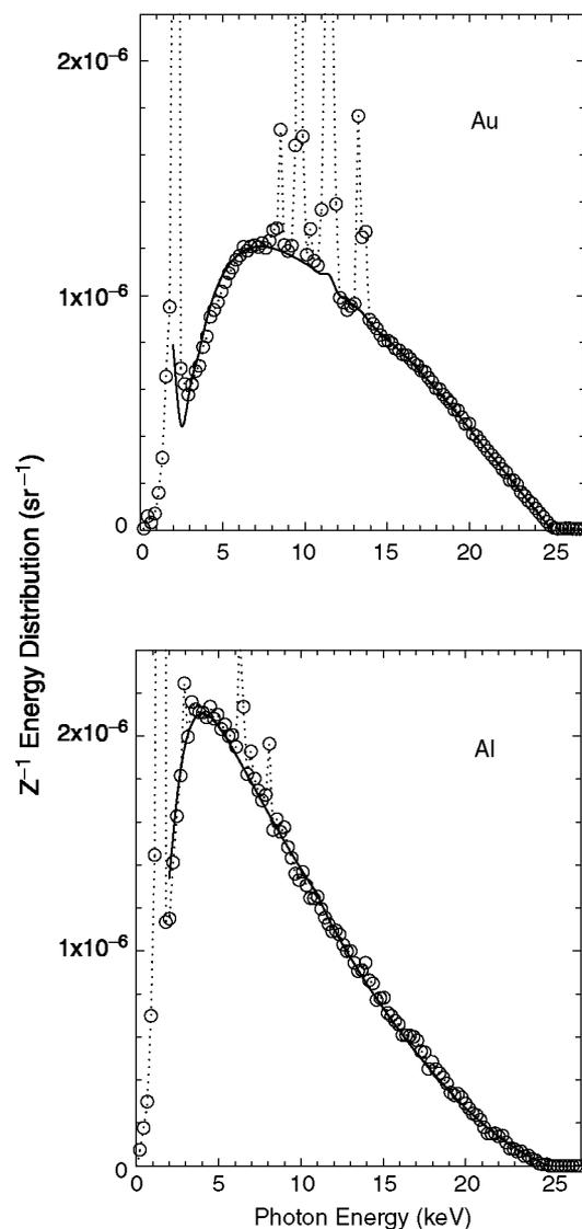
**Figure 5.** Illustration of the improved fit using the 'hybrid' model that switches from a fixed emission angle of 130° to an average emission angle at 0.4 times the incident electron energy. The improvement in the fit is more evident for the Al case when compared with Fig. 1, but there is also improvement in the Au fit, especially just below the L characteristic x-rays.
