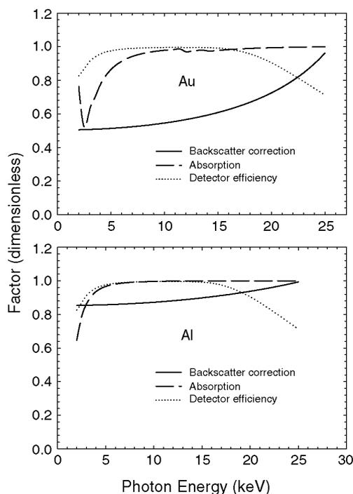
**Figure 4.** The backscattering correction factor, self-absorption correction factor and detector efficiency for Au and Al for 25 keV electrons.
