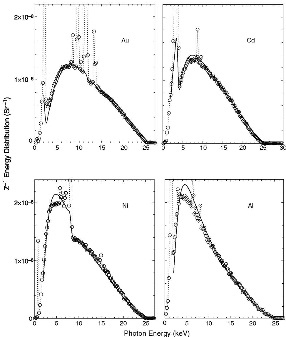
**Figure 1.** Typical results for the x-ray energy distribution from Eqn (4) in units of  $\text{sr}^{-1}$  for 25 keV electrons on targets of Au, Cd, Ni and Al. The data have been normalized to the model.
