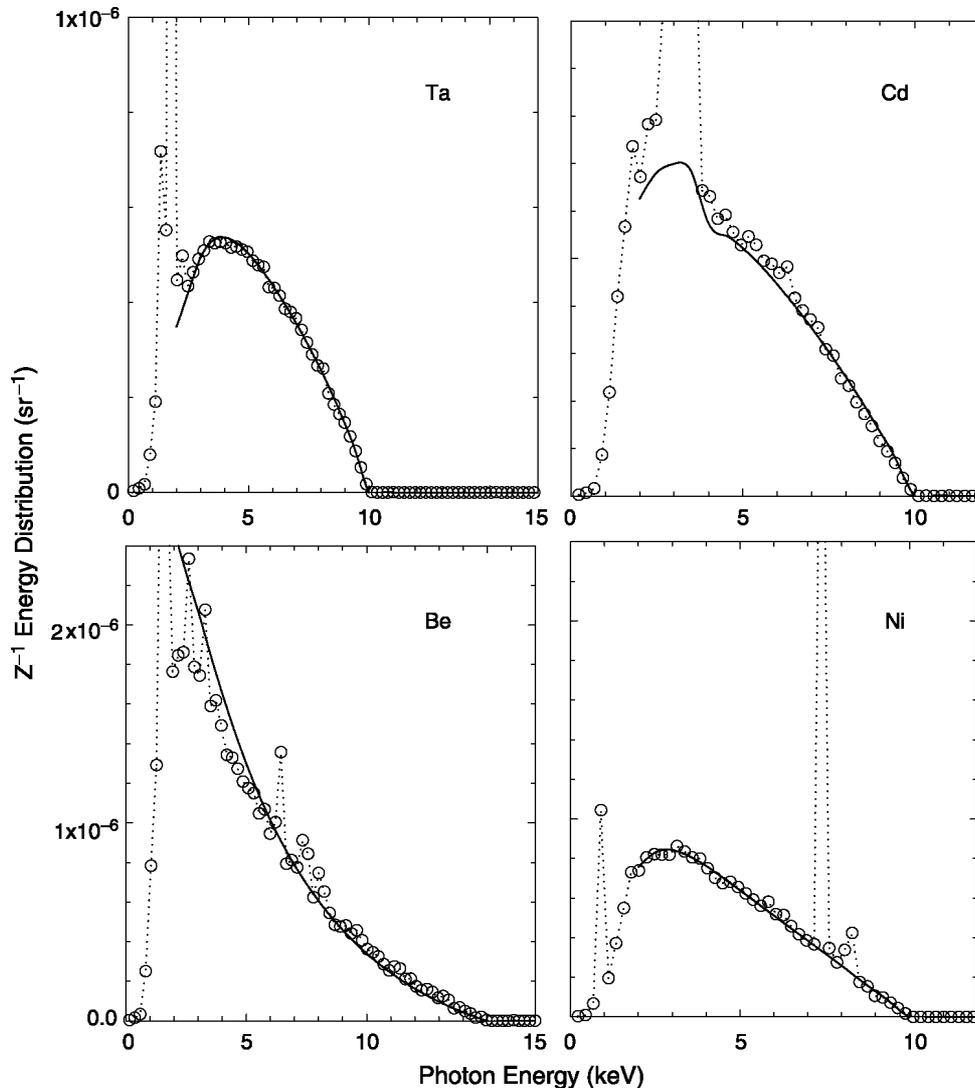
**Figure 2.** Typical results for the x-ray energy distribution from Eqn (4) in units of  $\text{sr}^{-1}$  for 10 and 15 keV electrons on targets of Ta, Cd, Ni and Be. The data have been normalized to the model.
