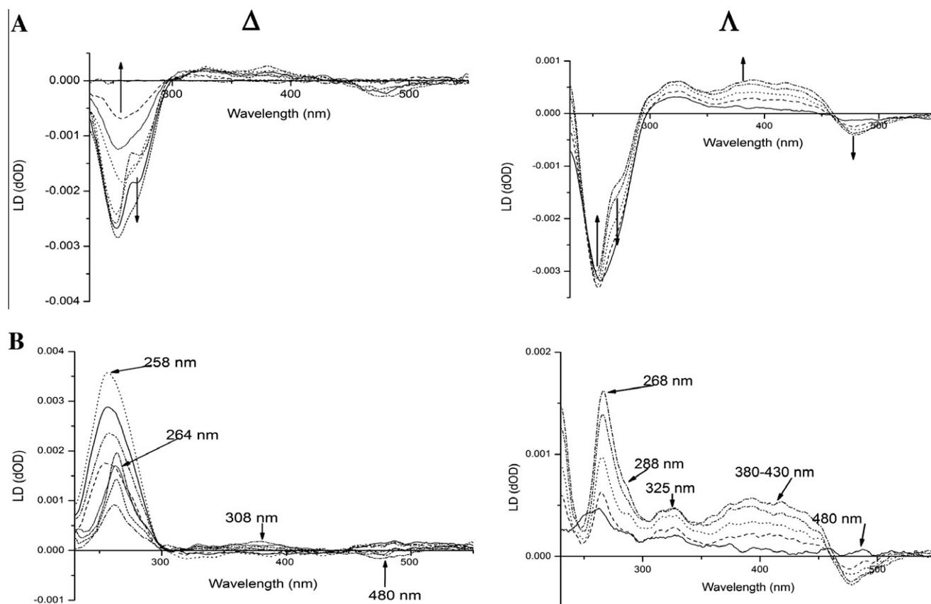
**Fig. 10.** (A) LD spectra of LD-DNA titration with  $\Delta$ -RUP1 (left) and  $\Lambda$ -RUP1 (right). (B) LD spectra where the DNA spectrum has been subtracted from each LD-DNA titration spectrum of  $\Delta$ -RUP1 (left) and  $\Lambda$ -RUP1 (right). The wavelength (nm) is plotted on the X-axis, while the MC complex concentration (M) on the Y- and the LD (dOD) on the Z-axis respectively.
