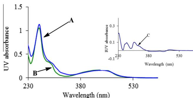
Fig. 8. The UV-Vis spectrum of RUP1 (A) and  $\text{rac-}[\text{Ru}(\text{phen})_2(\text{dpq})]^{2+}$  (B) the insert shows a spectrum where UV (B) is subtracted from UV (A) this represents the polyamide contribution to the spectrum (C) in  $\text{H}_2\text{O}$ :acetonitrile (1:1 v/v) mixture at room temperature. The concentration of both complexes was 10  $\mu\text{M}$ .
