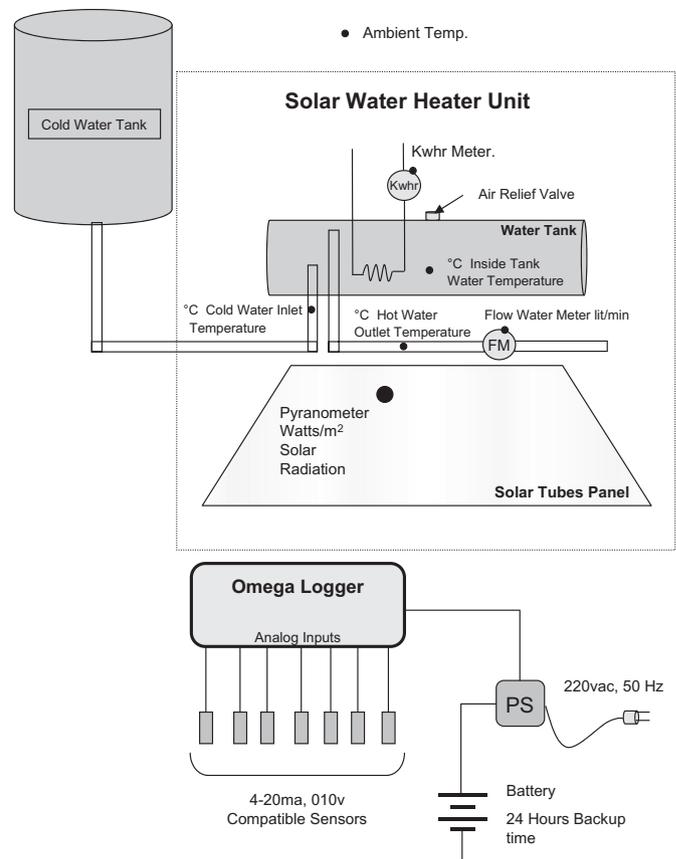
Scheme 1. Schematic of the monitoring equipment placement.
