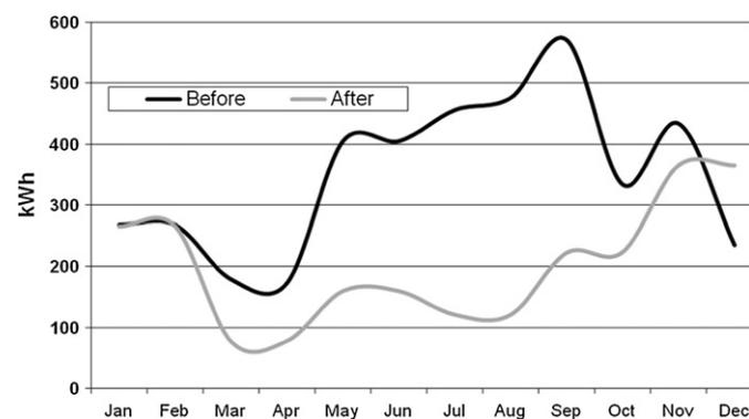
Fig. 1. Plot of electricity consumption (kWh) before and after SWH system installation.
