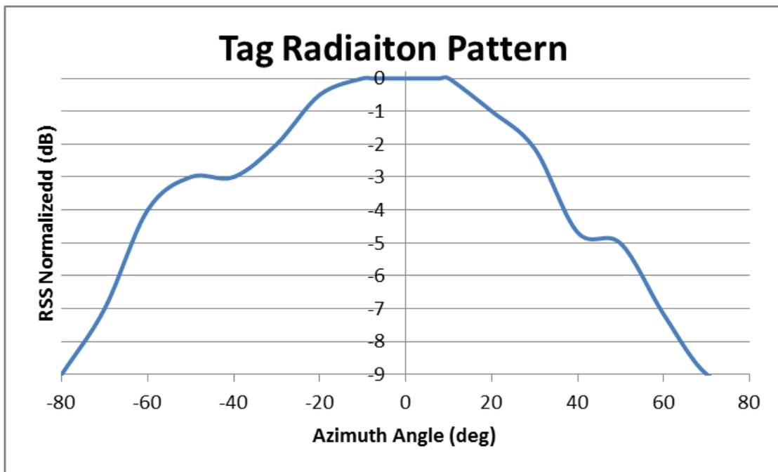
Figure 6. Tag's Antenna Radiation pattern
