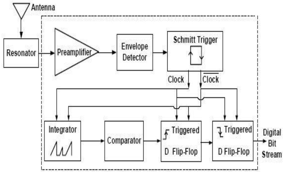
Figure 4. Demodulation stage
