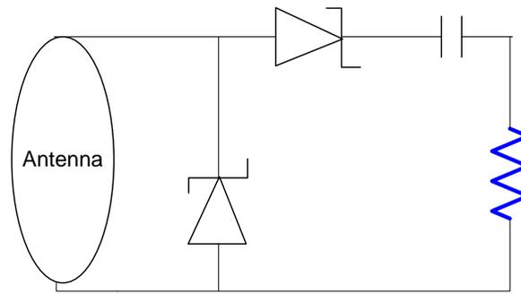
Figure 3.Schematic of Rectifying Circuit
