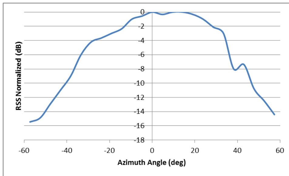
Figure 5. Reader's Antenna Radiation pattern
