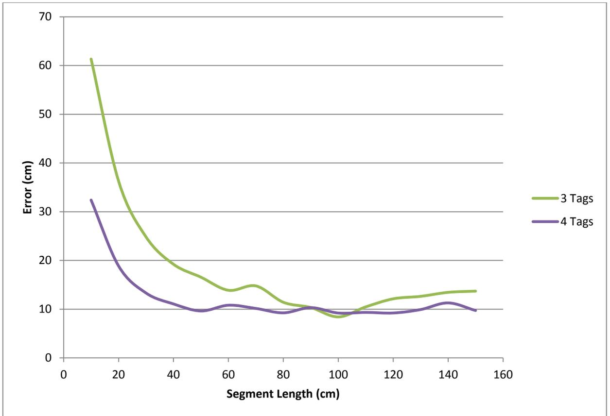
Figure 12. Error (cm) vs. Segment length (cm) for different tag configurations
