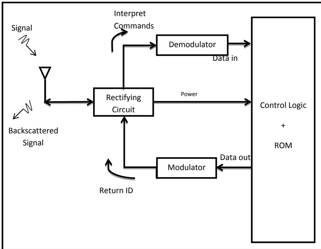
Figure 2. Schematic of a Passive RFID Tag
