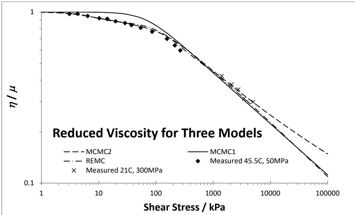
Figure 5. Comparing the MCMC1, MCMC2 and REMC models. MCMC1 eliminates the contribution from the higher molecular weight component.
