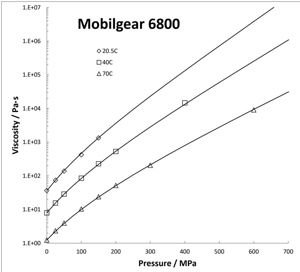
Figure 3. Measured low-shear viscosities and the improved Yasutomi correlation as the curves.
