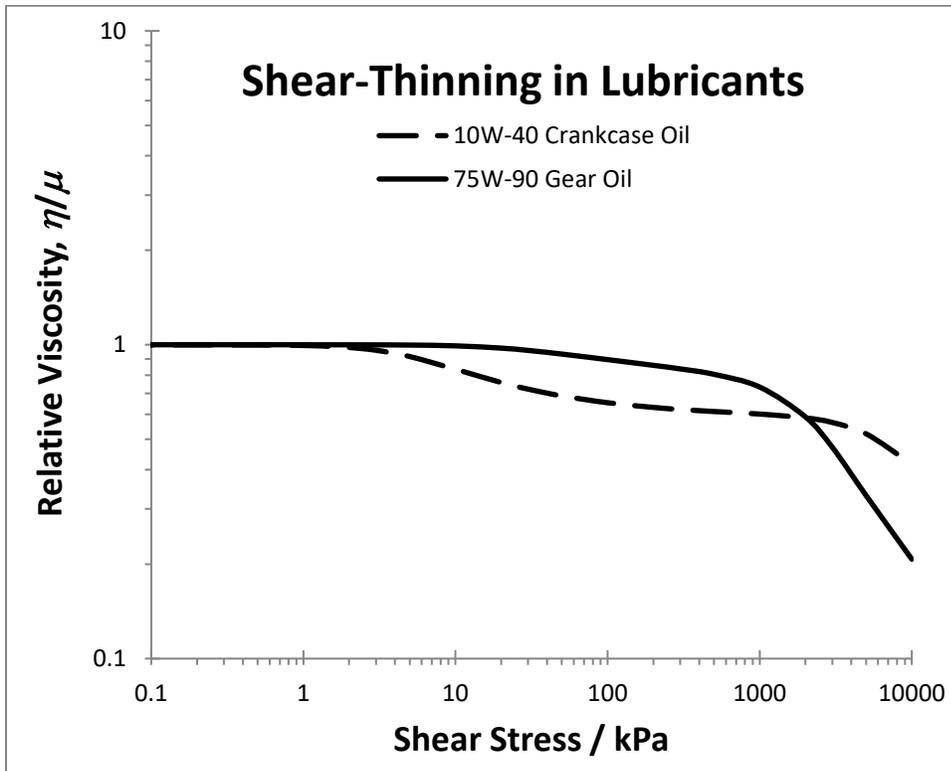
Figure 1. Shear-dependence of viscosity (flow curves) for a crankcase oil and a gear oil showing typical differences.
