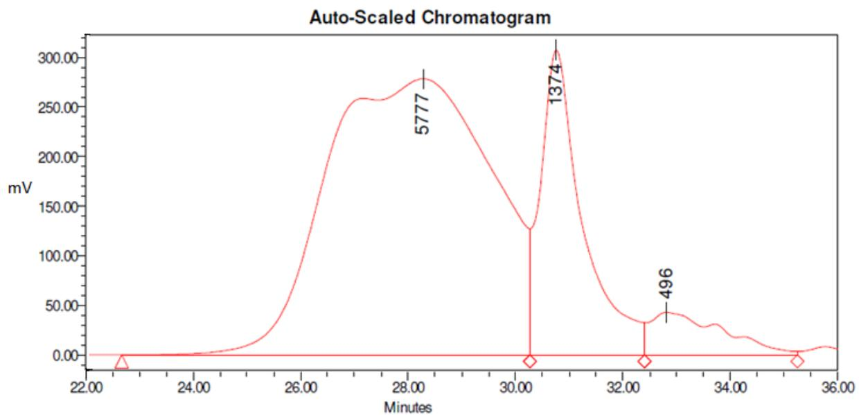
Figure 7. Chromatogram for Mobilgear SHC 6800. Molecular weights at peaks are given in Daltons.
