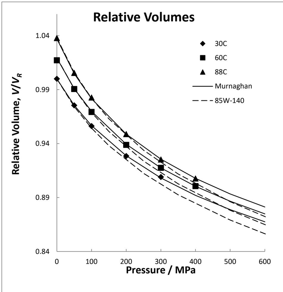
Figure 2. The measured relative volume compared with the Murnaghan equation and an 85W-140 gear oil.
