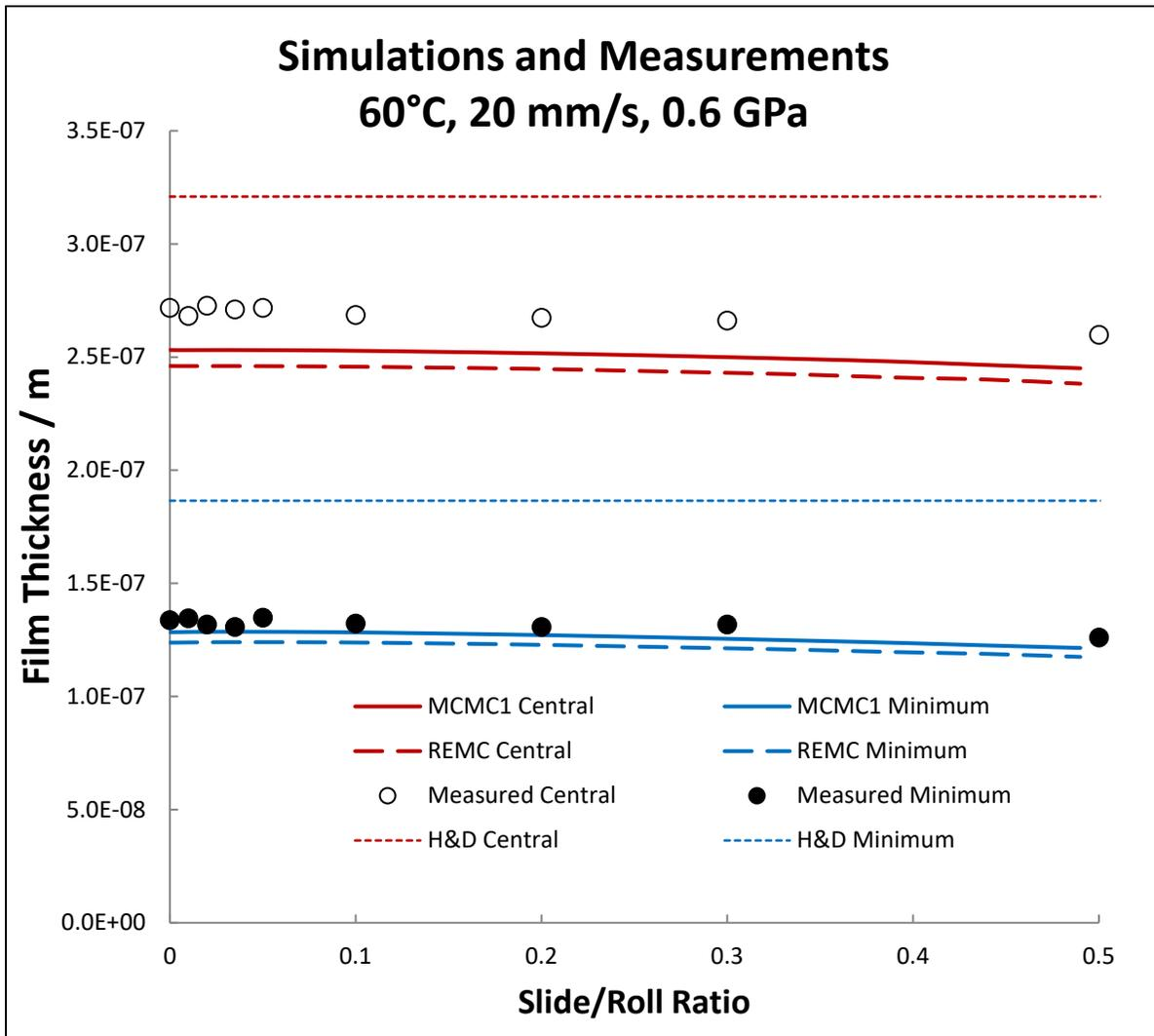
Figure 6. Film thickness measurements(ball moving faster than disk), calculated values and the Hamrock-Dowson **isothermal**, **Newtonian** predictions. Calculated curves obtained by the numerical solution described in Section 6 are provided for two shear-thinning models.
