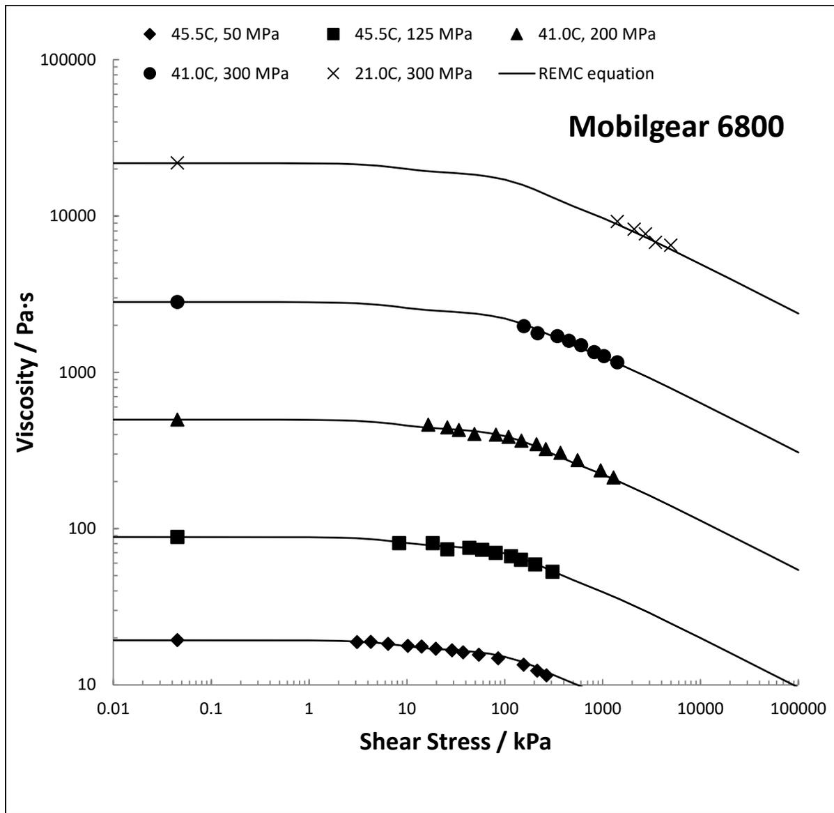
Figure 4. Measured shear-dependent viscosities. Curves are the REMC model.
