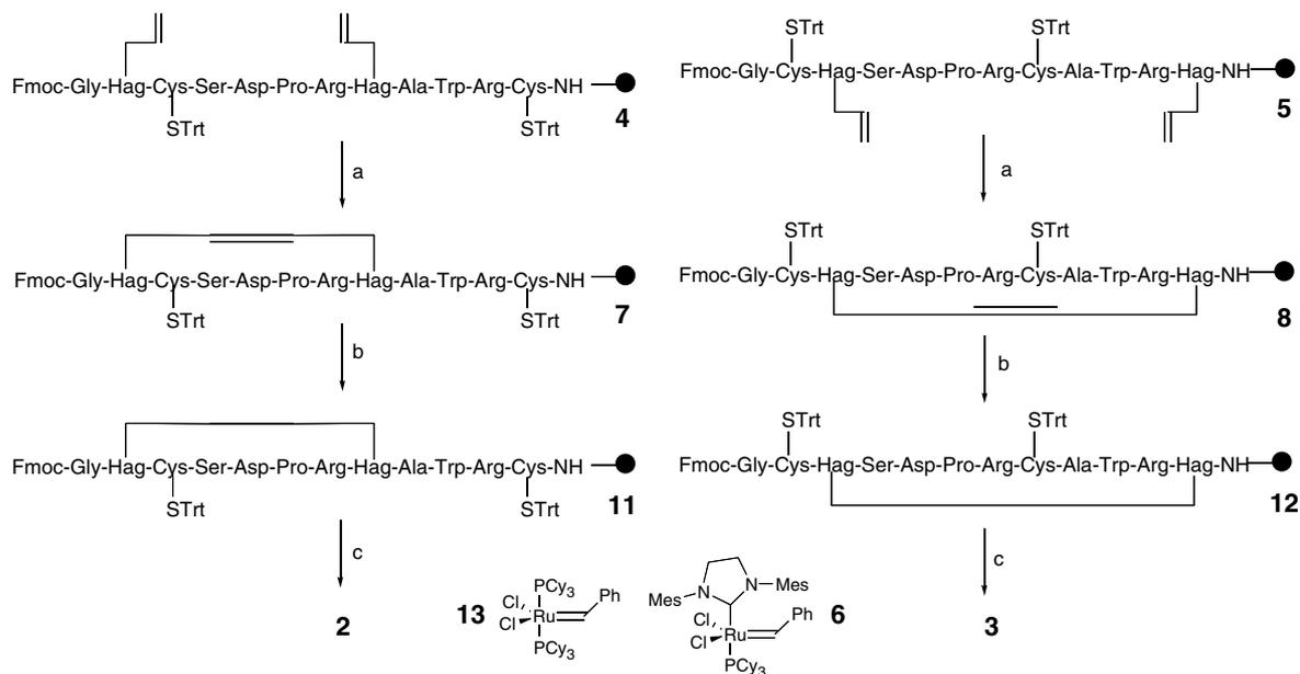
**Scheme 2** Reagents and conditions: Rink amide resin (●, 0.52 mmol/g loading). (a) 5–10 mol% second-generation Grubbs' catalyst, DCM-10% 0.4 M LiCl/DMF, rt  $\rightarrow$  100 °C, 1–2 h, microwave irradiation; (b) Rh(I)(PPh<sub>3</sub>)<sub>3</sub>Cl, 80 psi H<sub>2</sub>, rt, 10% MeOH in DCM, 14 h; (c) Fmoc-de-protection and resin cleavage.
