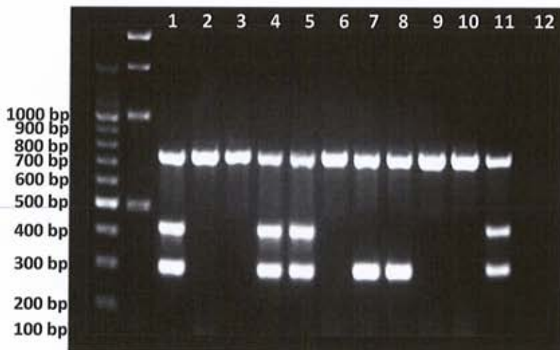
Fig 1. 1.5% agarose gel electrophoresis showing representative PCR products after 16S rRNA, PVL and mecA amplification. The first and the second lanes show DNA marker 100bp and 500bp (Fermentas) lanes 1-11 show PCR products of the three genes of different isolates. Lane 12 is the negative control.
