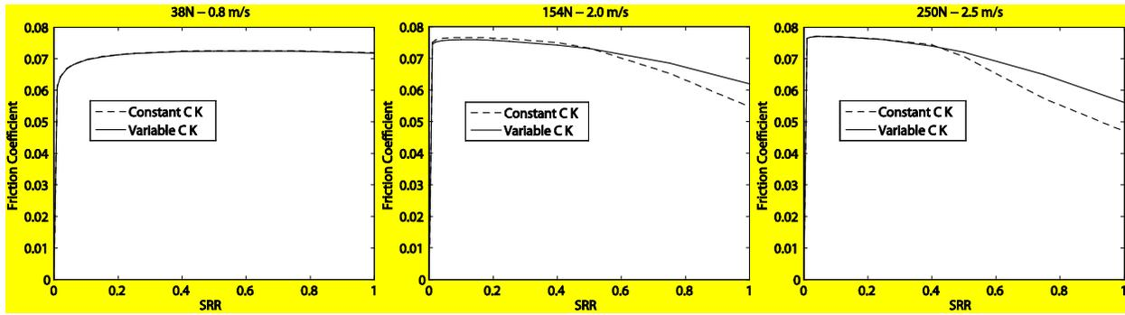
**Figure 8:** Traction curves as a function of slide-to-roll ratio (*SRR*) for a steel-steel circular contact under loading and mean entrainment speed conditions of test cases A, B and C
