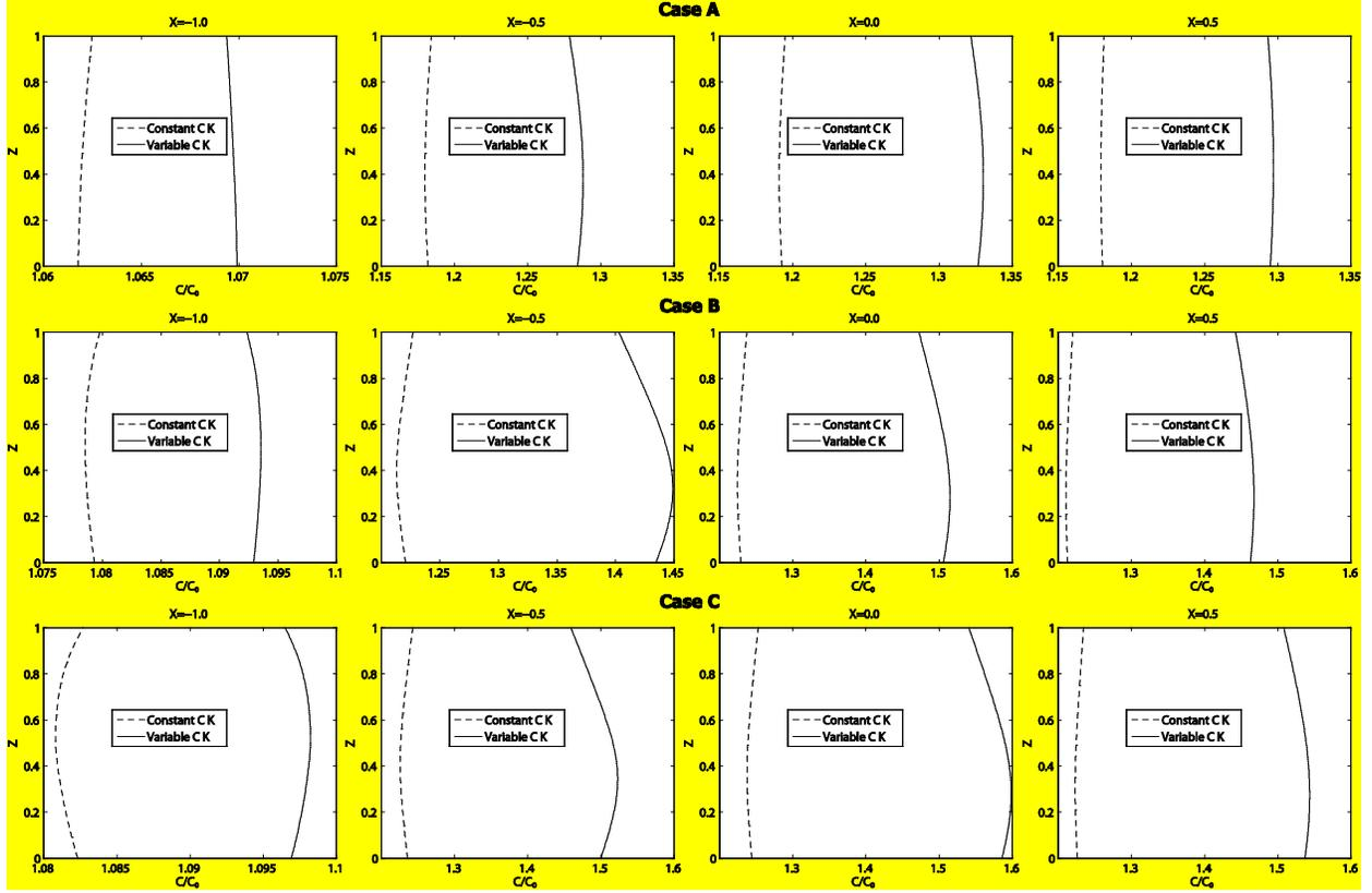
**Figure 2:** Volumetric heat capacity variations in the lubricant film thickness along the central line of the contact at different  $X$  locations
