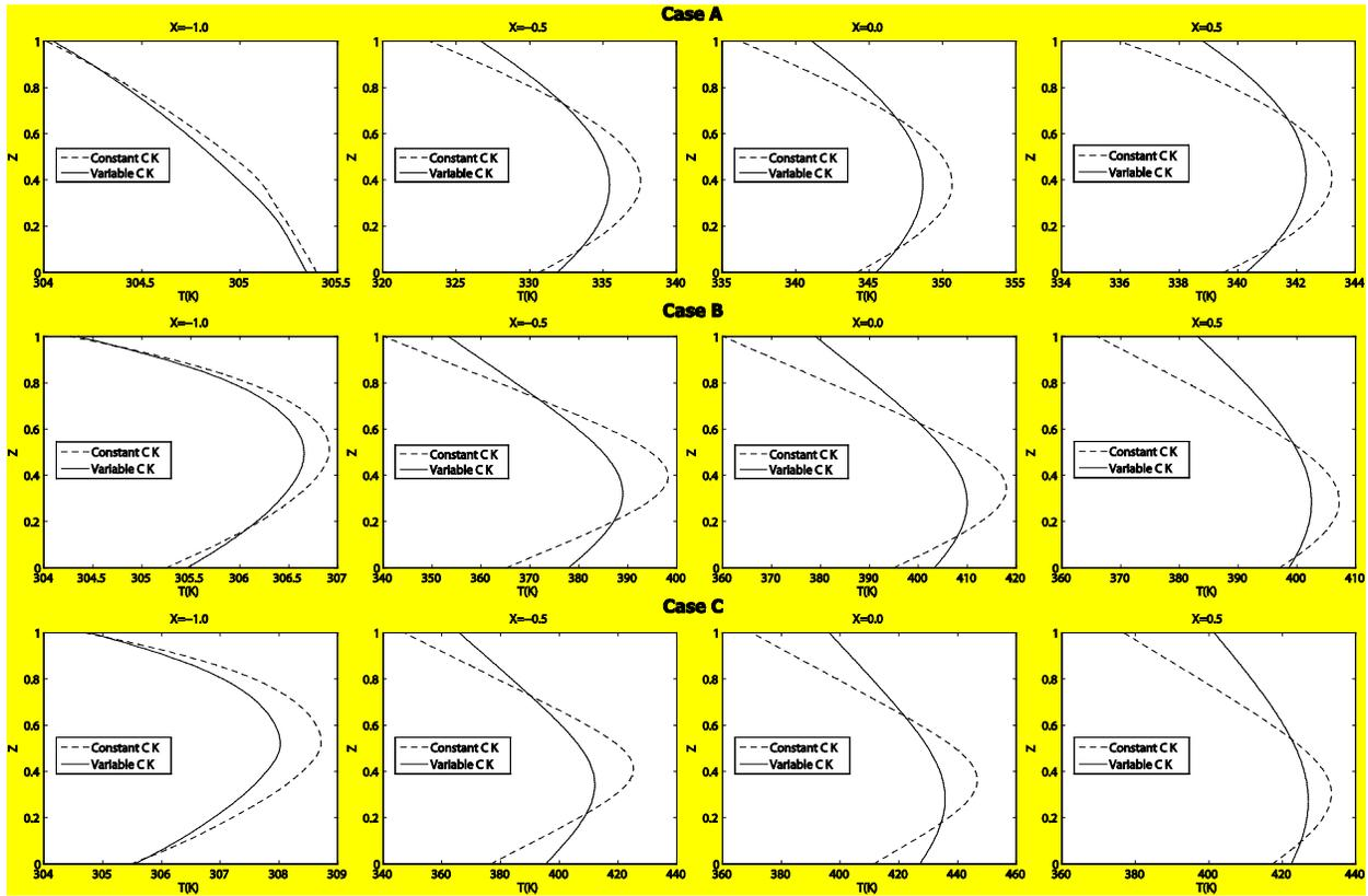
**Figure 3:** Temperature variations in the lubricant film thickness along the central line of the contact at different  $X$  locations
