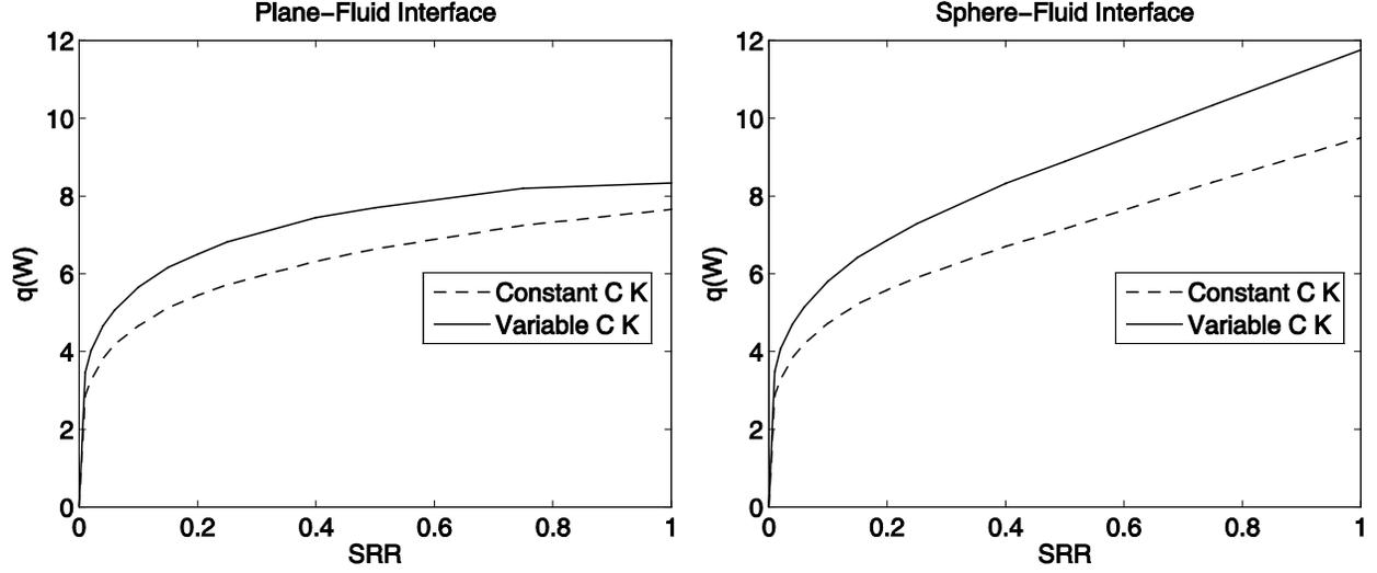
**Figure 6:** Heat flux variations as a function of *SRR* at the solid-liquid interfaces for test case B
