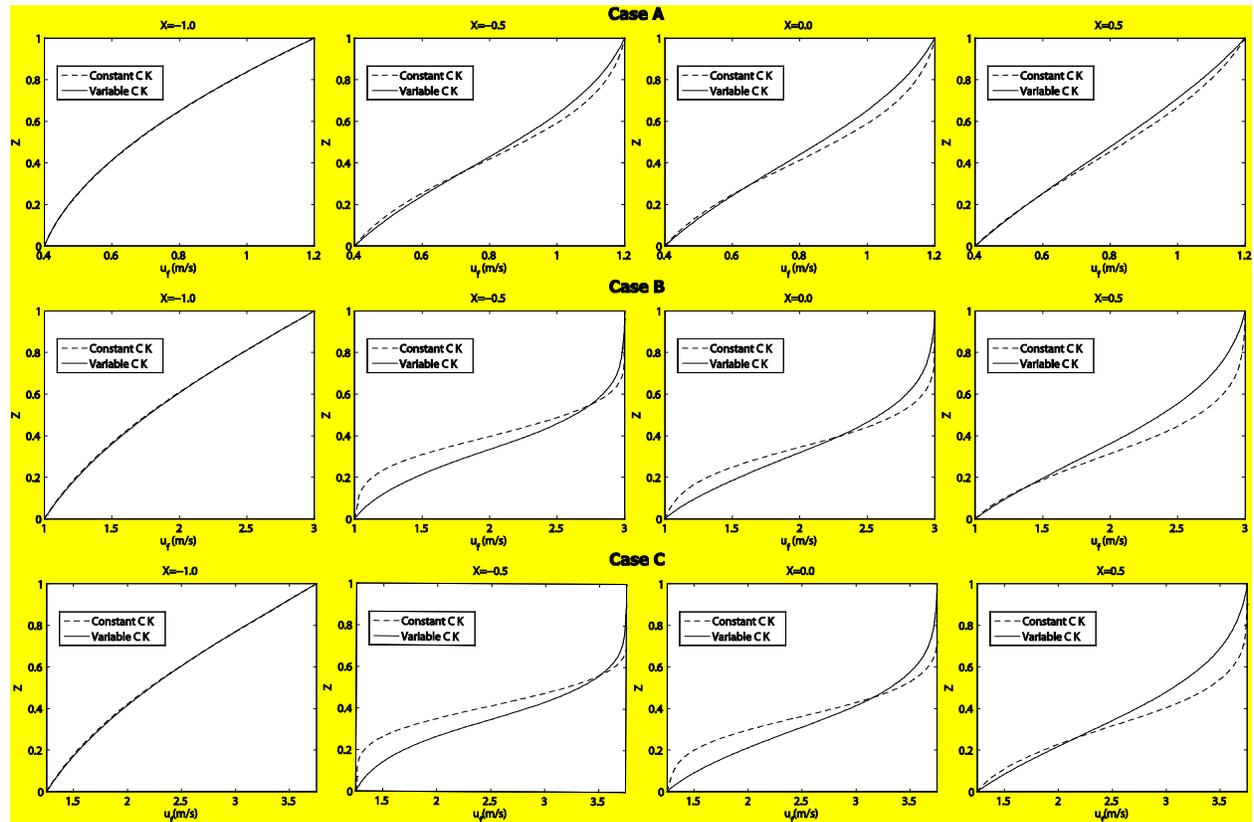
**Figure 5:** Lubricant flow  $x$ -velocity component  $u_f$  variations in the lubricant film thickness along the central line of the contact at different  $X$  locations
