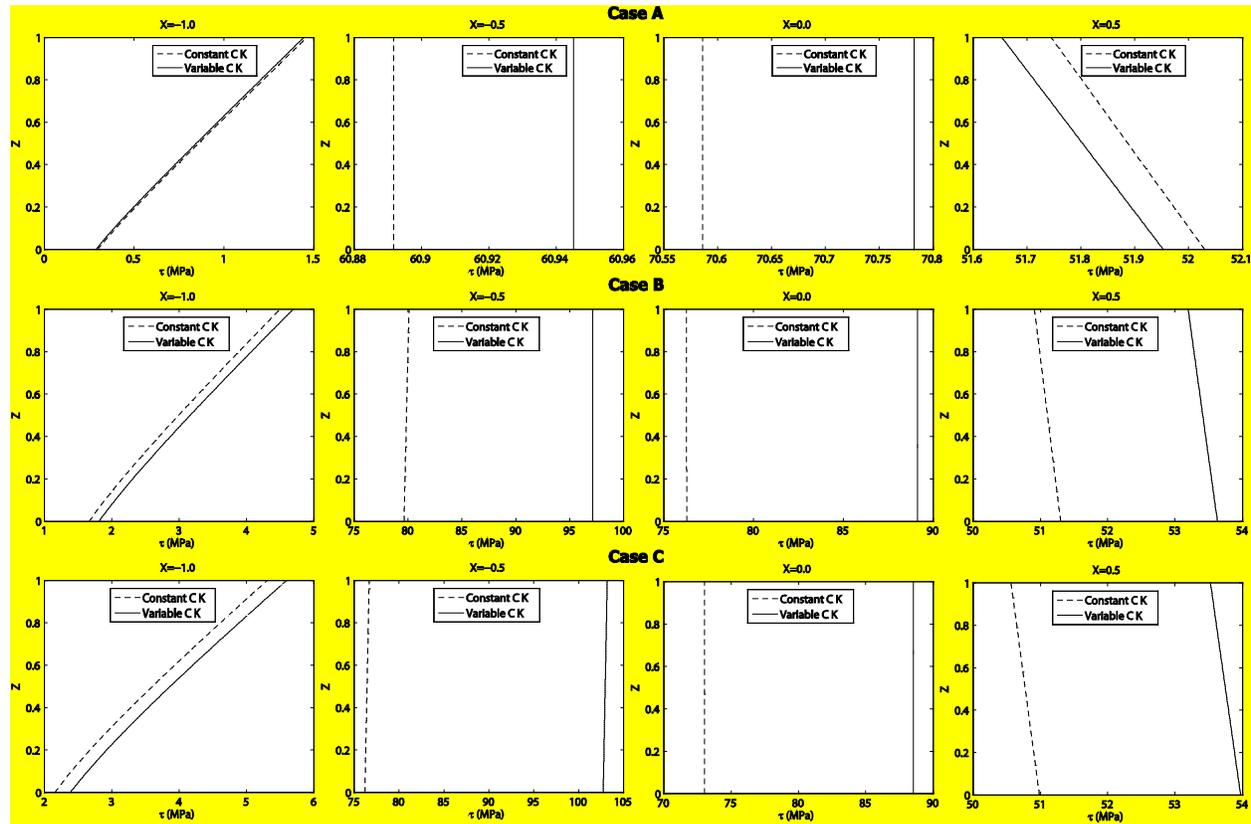
**Figure 7:** Shear stress variations in the lubricant film thickness along the central line of the contact at different  $X$  locations
