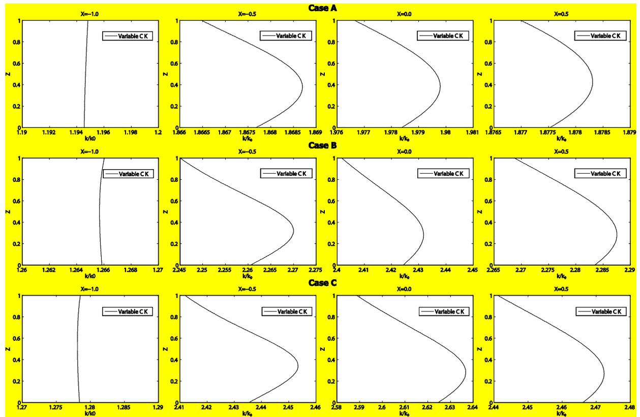
Figure 1: Thermal conductivity variations in the lubricant film thickness along the central line of the contact at different X locations
