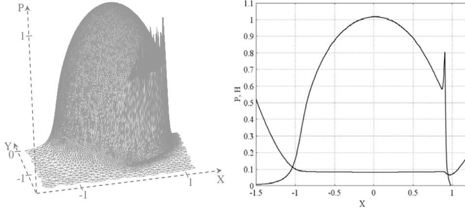
**Figure 8:** 3D dimensionless pressure profile (Left), dimensionless pressure and film thickness profiles along the central line in the  $X$ -direction (Right) ( $F=100\text{N}$ ,  $p_h=1\text{ GPa}$ ,  $u_1=u_2=0.8\text{ m/s}$ ,  $R=16\text{ mm}$ ,  $\mu_R=0.04\text{ Pa}\cdot\text{s}$ ,  $\alpha=22\text{ GPa}^{-1}$  and  $T=T_0=T_R=20\text{ }^\circ\text{C}$ )
