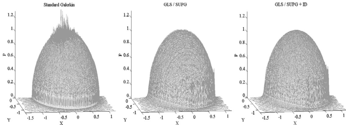
**Figure 12:** Stabilization effects on circular thermal EHD contacts ( $F=1000$  N,  $p_h=1.66$  GPa,  $\alpha^*=18.53$  GPa $^{-1}$ ,  $u_1=u_2=1$  m/s,  $R=12.7$  mm)
