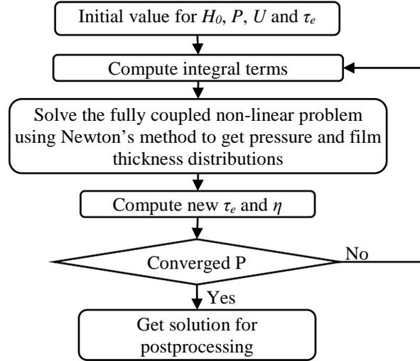
**Figure 11:** flow diagram for the numerical modelling of an isothermal EHL circular contact lubricated with a non-Newtonian lubricant
