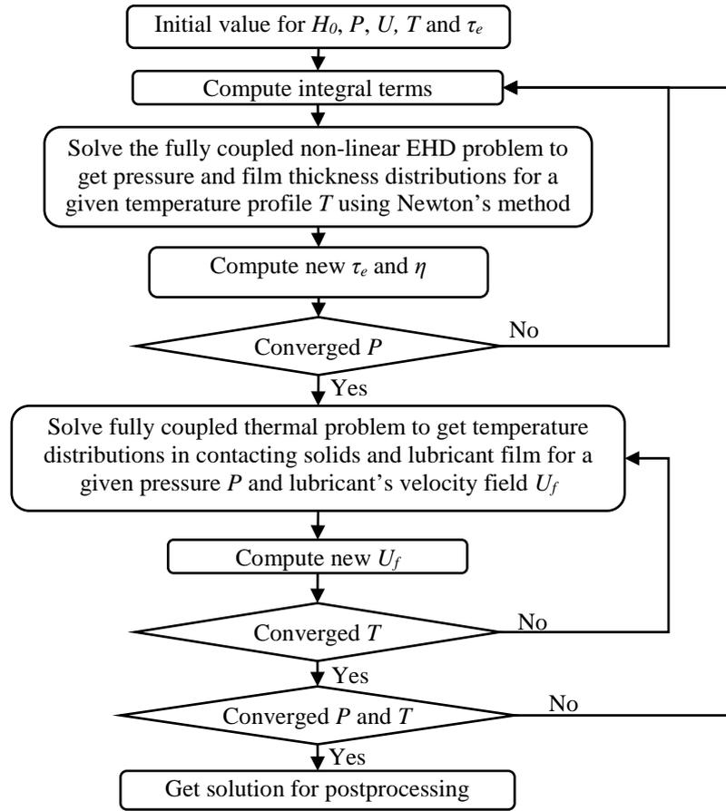
**Figure 13:** Flow diagram of the thermal EHL (TEHL) model
