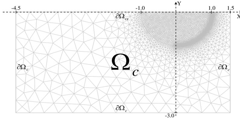
**Figure 7:** Meshing of the contact area  $\Omega_c$
