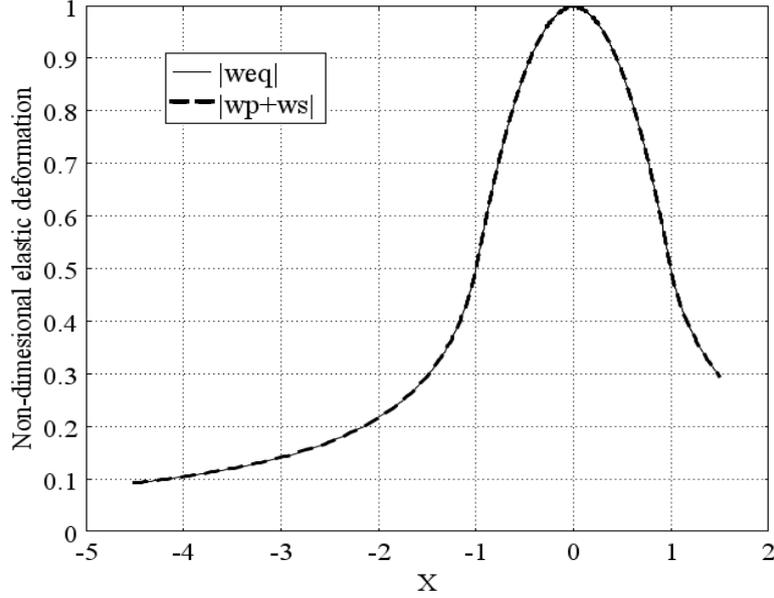
**Figure B.2:** Total elastic deflection of a dry glass-on-steel circular contact
