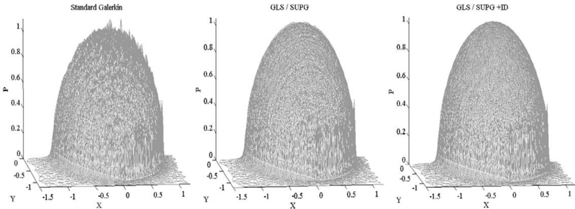
**Figure 10:** Stabilization effects on circular EHD contacts lubricated with a non-Newtonian lubricant ( $F=1000$  N,  $p_h=1.66$  GPa,  $\alpha^*=18.53$  GPa $^{-1}$ ,  $u_1=u_2=1$  m/s,  $R=12.7$  mm,  $T=T_0=T_R=40$  °C)
