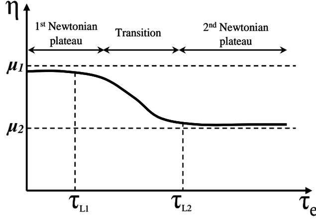
**Figure 9:** Typical behaviour of a non-Newtonian lubricant modelled by the Carreau model
