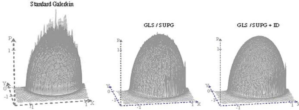
**Figure 5:** Heavily loaded circular contact problem and the effect of stabilization. Left: Standard Galerkin, Centre: SUPG/GLS, Right: SUPG/GLS+ID ( $p_h=3$  GPa,  $\mu_R=0.012$  Pa.s,  $\alpha^*=23$  GPa $^{-1}$ ,  $u_1=u_2=1$  m/s,  $R=12.7$  mm,  $A_1=19.17$  °C,  $A_2=4.07 \times 10^{-3}$  MPa $^{-1}$ ,  $B_1=0.23$ ,  $B_2=0.0249$  MPa $^{-1}$ ,  $C_1=16.04$ ,  $C_2=18.18$  °C,  $T_g(0)=-73.86$  °C,  $\mu_g=10^{12}$  Pa.s and  $T=40$  °C)
