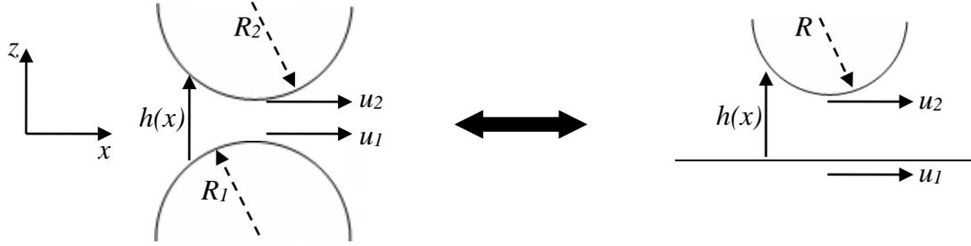
**Figure 1:** EHL line contact and the equivalent reduced geometry
