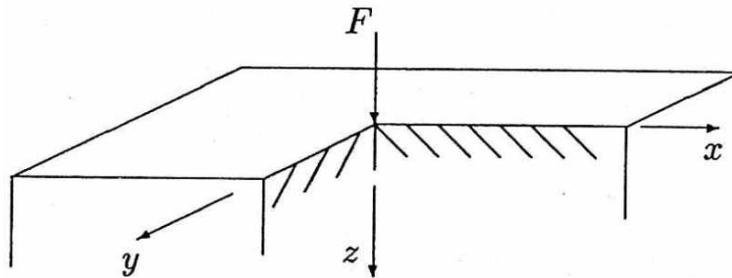
**Figure B.1:** Point loading of an elastic half space
