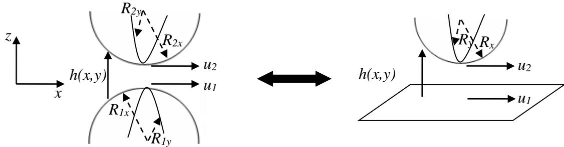
**Figure 2:** EHL point contact and the equivalent reduced geometry
