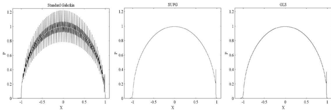
**Figure 4:** Heavily loaded line contact problem and the effect of stabilization. Left: Standard Galerkin, Centre: SUPG, Right: GLS ( $p_h=3$  GPa,  $\mu_R=0.012$  Pa.s,  $\alpha^*=23$  GPa $^{-1}$ ,  $u_1=u_2=1$  m/s,  $R=15$  mm,  $A_1=19.17$  °C,  $A_2=4.07 \times 10^{-3}$  MPa $^{-1}$ ,  $B_1=0.23$ ,  $B_2=0.0249$  MPa $^{-1}$ ,  $C_1=16.04$ ,  $C_2=18.18$  °C,  $T_g(0)=-73.86$  °C,  $\mu_g=10^{12}$  Pa.s and  $T=40$  °C)
