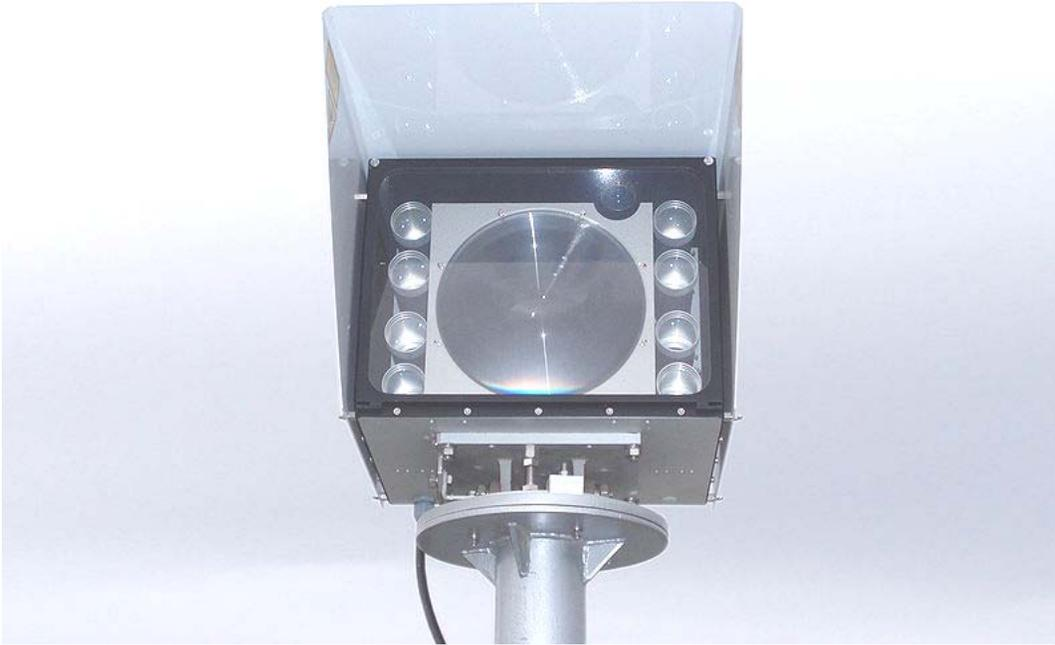
**Figure 4: An 8-beam free space optics laser link. The receiver is the large disc in the middle, the transmitters the smaller ones. To the top and right side a monocular for assisting the alignment of the two heads**
