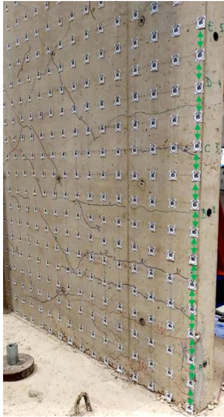
Fig. 32 Strain readings between targets at the web edge
