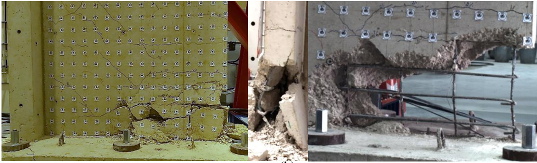
(a) (b) (c) Fig. 10 As-built wall (W) at the end of the test, after failure
