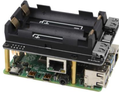
Figure 43: Makerhawk Battery Module [38]
