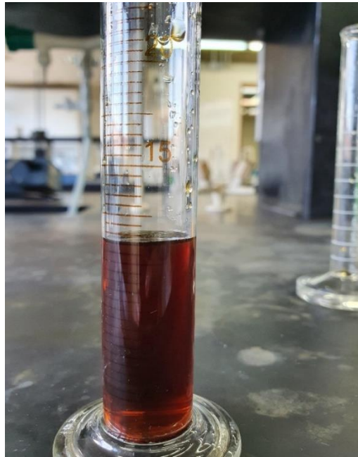
Figure 12 - 5.3 ml Black Maca liquid extract after rotary evaporation
