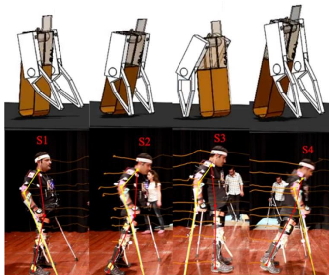
Figure 4 - Side by side comparison of simulation and experimental models.
