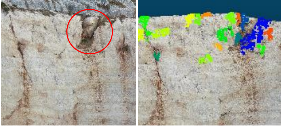
Figure 14: Joints successfully detected using DSE and viewed in CloudCompare
