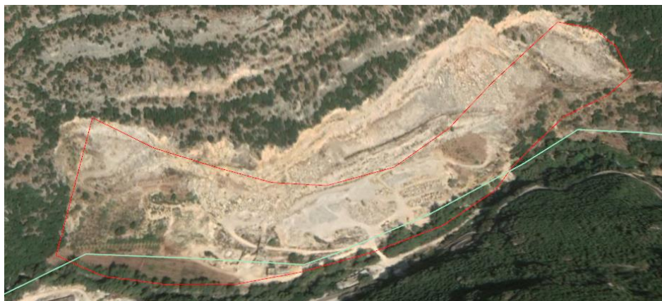
Figure 35: Variation between available polygon layer of quarries' area and actual quarry in Google Earth
