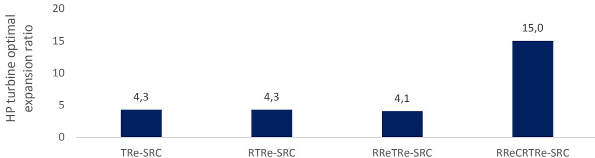
Fig. 4. High pressure turbine optimal expansion ratio for the different turbine reheat systems.
