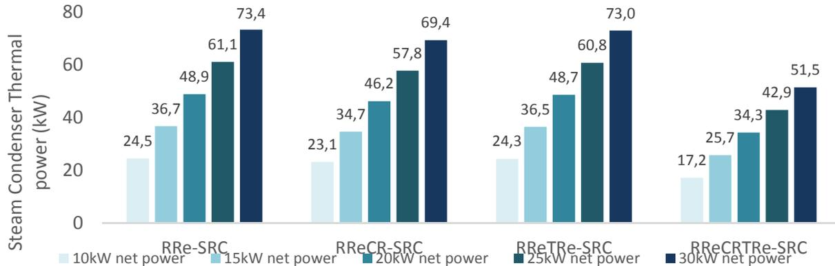
Fig. 5. Steam condenser thermal power function of net mechanical power for the different selected VCM-machines.
