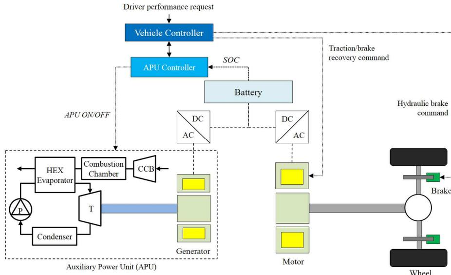
Fig. 1. Configuration of the modelled SHEV with a simple VCM APU.
