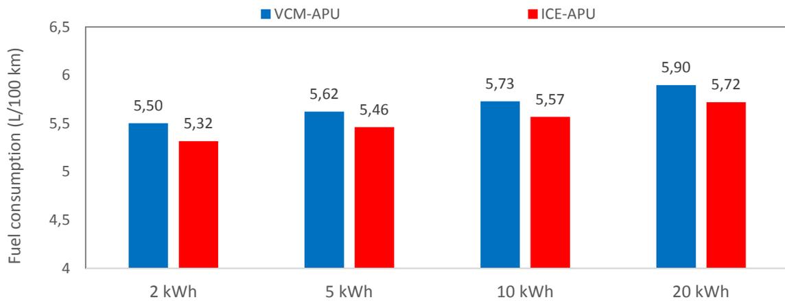
Fig. 7. Fuel consumption of VCM-APU and ICE-APU for the different battery capacities
