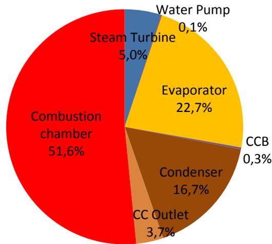
*Fig. 2. Distribution of exergy destruction in the SRC system with maximum combustion chamber temperature of 1250°C and maximum cycle pressure of 10 MPa.*
