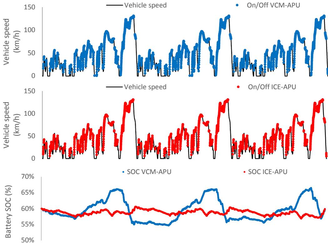
Fig. 6. Results emulating SHEV with 5 kWh battery on 3 WLTC (SOC<sub>i</sub> = SOC<sub>f</sub> = 60%).
