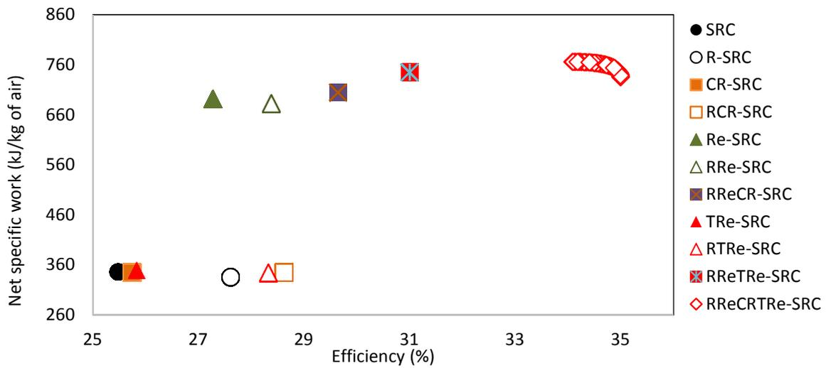
Fig. 3. Pareto optimal efficiencies and net specific work solutions of the different VCM-systems.
