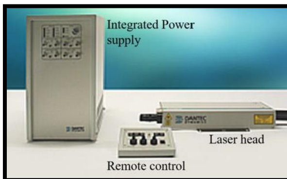
Figure 99: A PIV Power Supply and Control Unit
