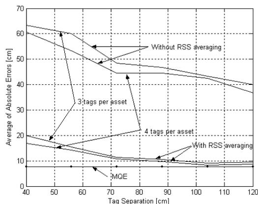
Fig. 3. Mean absolute errors versus tag separation
