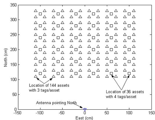
Fig. 6. Location of antenna and distribution of objects with tag separation = 40 cm
