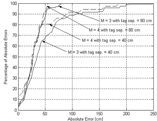
Fig. 7. CD of *position* errors for the case of three- and four-tag deployment with tag separation equal to 40 cm and 80 cm
