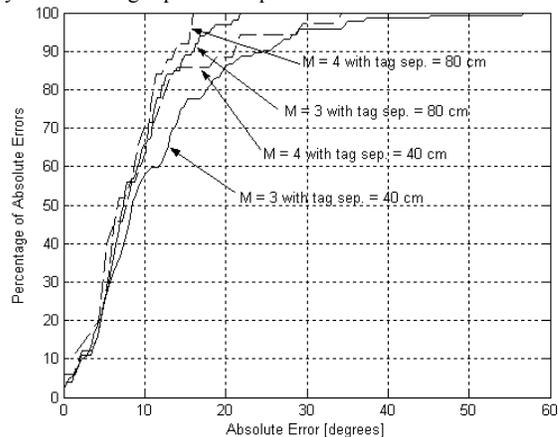
Fig. 8. CD of *orientation* errors for the case of three- and four-tag deployment with tag separation equal to 40 cm and 80 cm
