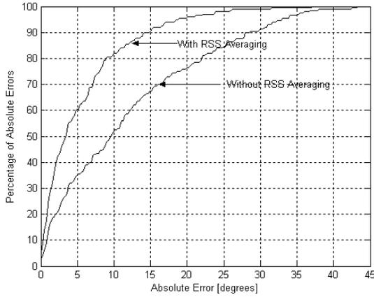
Fig. 5. Cumulative distribution of orientation errors for the case of three-tag deployment and with tag separation = 80 cm
