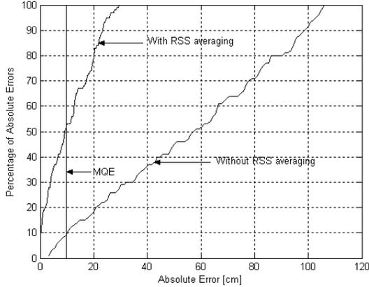
Fig. 4. Cumulative distribution of position errors for the case of three-tag deployment and with tag separation = 80 cm
